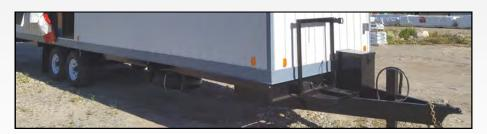
Tandem Wheel type suspension 2 X 7000 pounds axles, 16" Torque/flex wheels
